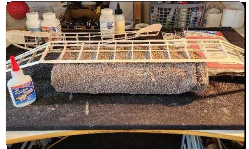
Wings ready for covering
